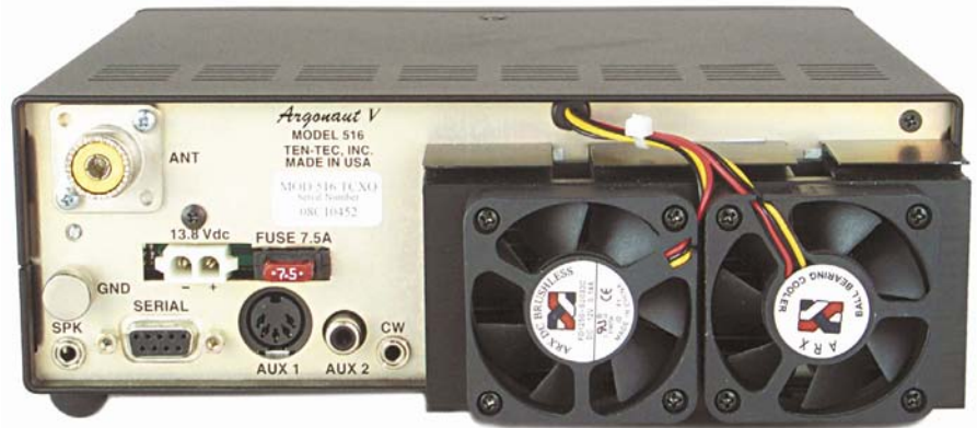
Figure 4—Rear panel of the Argonaut V. Note the sizeable cooling fans (right). Firmware updates are received through the SERIAL port (lower left). The Argonaut V and the computer may be connected with a standard 9-pin serial cable.
